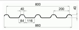
Straight ribbed sheet **R526** produced with polyester resin reinforced with fibreglass, in conformity to the following characteristics and technical norms:
