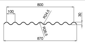
Straight corrugated sheet **R527** produced with polyester resin reinforced with fibreglass, in conformity to the following characteristics and technical norms:
