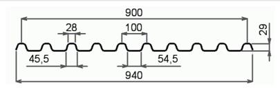
Straight ribbed sheet **R578** produced with polyester resin reinforced with fibreglass, in conformity to the following characteristics and technical norms:
